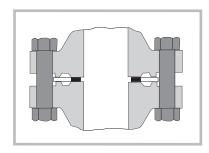
**CG-RJ** and **CGI-RJ** Spiral Wound Gaskets are designed for use, as a replacement maintenance item, of standard oval and octagonal ring joint gaskets. These gaskets are available for NPS ½ to 24 and pressure classes 150 to 1500. Gasket thickness is 0.175" (4.5mm) and the outer ring thickness is 0.125" (3.2mm).
