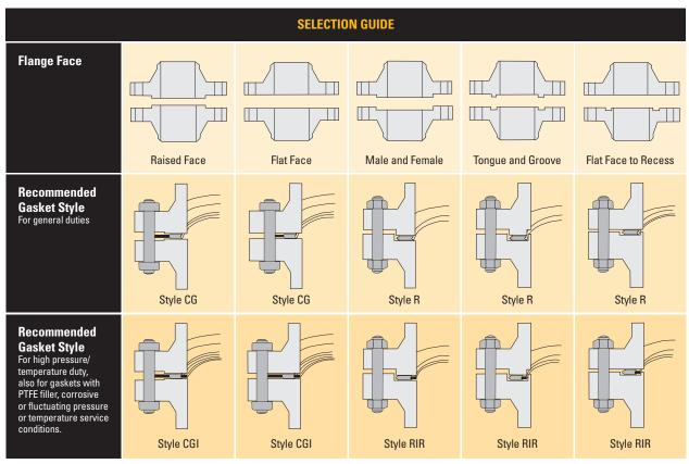
NOTES: Where style R gaskets are fitted it is essential that the flange is correctly dimensioned to provide a compression stop, as over compression can result in failure.
