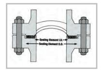
Standard Style R gaskets embody all the exclusive features of Flexitallic design for keeping compression values in balance with bolting and providing adequate resilience to compensate for variable stresses encountered in service. Standard Style R gaskets are manufactured to a nominal thickness of .125" (3.2mm). Optimum compression is in the range of .090" to .100" (2.3mm to 2.5mm) thick.
