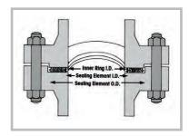
**Standard RIR** gaskets are manufactured to 0.125" (3.2mm) thickness. The gasket features a solid metal inner ring nominally 0.090" (2.3mm) thick, as an integrated part of its design. The inner ring provides a positive stop preventing the gasket from over compression and possible damage.
