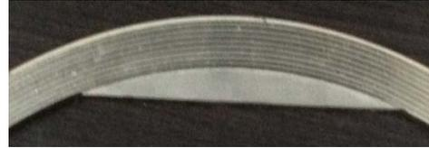
**Figure 12.** Photo of blade retainer
