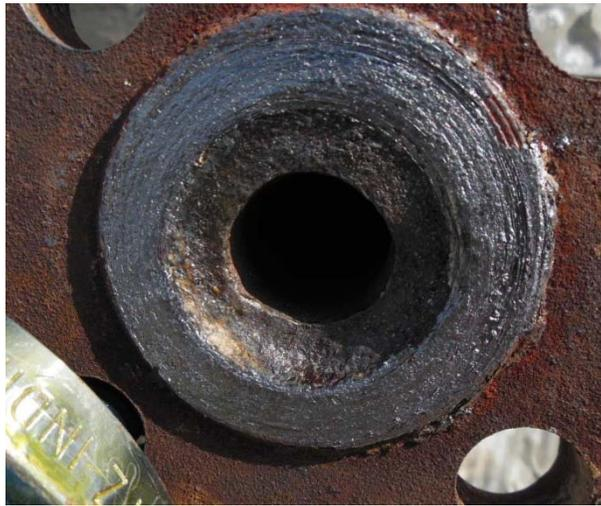
**Figure 14.** NPS 1" Class 150 SCH 160 Carbon steel flange corroded by HCl.
