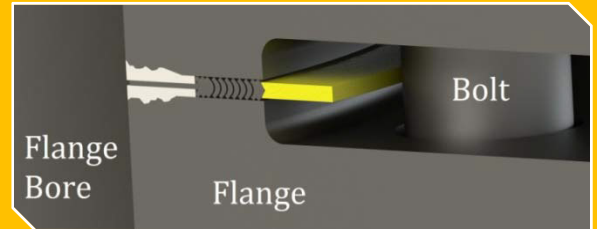
Change-HF™ Installed in a Corroded Flange
