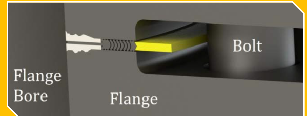
Change-HF™ Installed in a Corroded Flange
